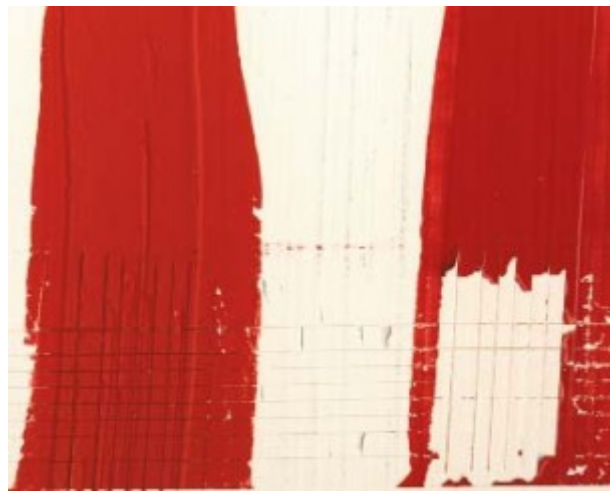
Cross Hatch Adhesion Test – Right: Oil paint is easily removed from a smooth ground. Left: Oil paint is adhered well to a toothy ground.
