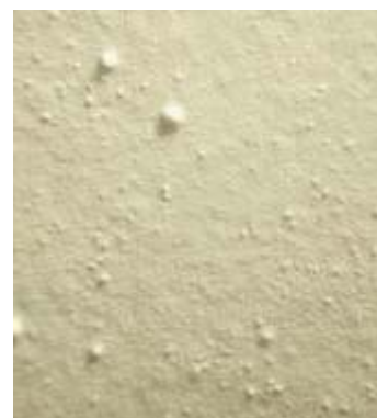
Random surface quality due to inconsistent particle size of pigment solids.
